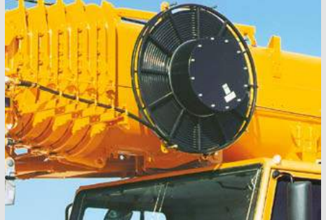
Hose reel for the hydraulic cylinder
