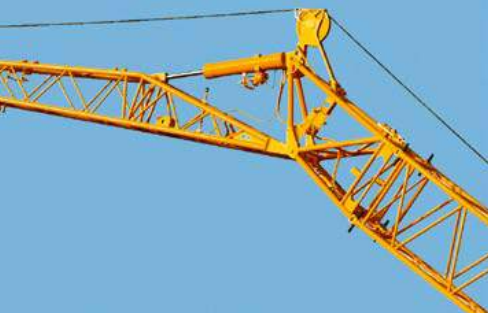
Hydraulically adjustable folding jib (0° to 40°)
